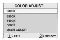
**9300K** — Adds blue to the screen image for cooler white (used in most office settings with fluorescent lighting).
